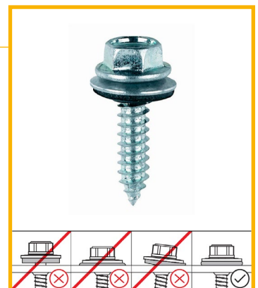
Self-Drilling Screw with EPDM Sealing Washer (8mm Socket)
